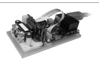
Figure 41. IS4920 EMI Test System
